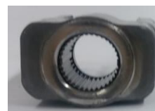
Fig. 1 Cold forged pinch yoke to be studied
