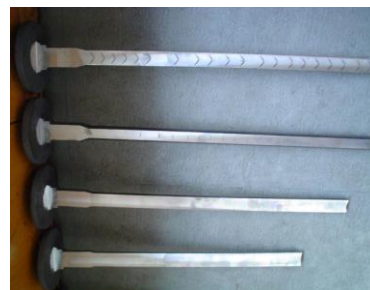
Fig. 1. Experimental chevron defects found in open-die extrusion process
